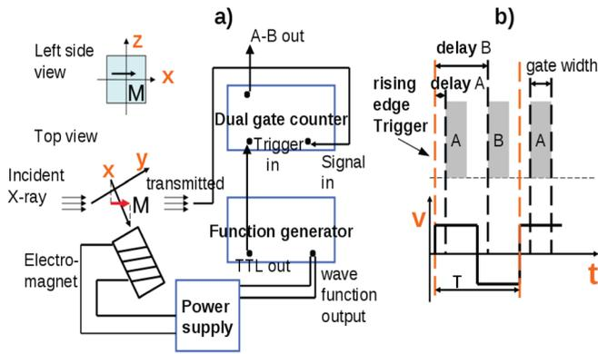
FIG. 1. (Color online) Experimental setup at CLS 10ID-1. (a) Configuration of the incident x-ray beam, sample plane, and photon detector; equipment setup for photon counter and function generator. (b) The wave function, trigger signal, and configurations for the 2 counting gates. See the text for details.
