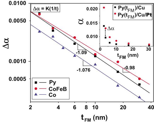
FIG. 3. (Color online) *Inset*:  $\alpha_{\text{nopT}}(t_{\text{FM}})$  and  $\alpha_{\text{Pt}}$  for Py after linear fits to data in Fig. 2. *Main panel*:  $\Delta\alpha(t_{\text{FM}}) = \alpha_{\text{Pt}}(t_{\text{FM}}) - \alpha_{\text{nopT}}(t_{\text{FM}})$  for Py, CoFeB, and Co. The slopes express the power law exponent  $n = -1.04 \pm 0.06$ .
