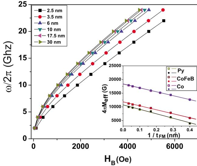
FIG. 1. (Color online) Fields for resonance  $\omega(H_B)$  for in-plane FMR, FM =  $\text{Ni}_{81}\text{Fe}_{19}$ ,  $2.5 \text{ nm} \leq t_{FM} \leq 30.0 \text{ nm}$ ; solid lines are Kittel fits. *Inset*:  $4\pi M_s^{\text{eff}}$  for all three FM/Cu, with (filled circles) and without (open squares) Pt overlayers.
