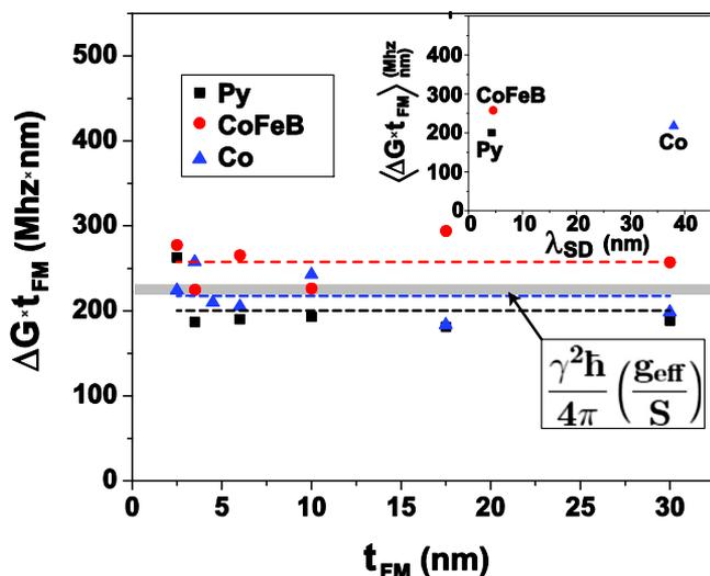
FIG. 4. (Color online) The additional nonlocal relaxation due to Pt overlayers, expressed as a Gilbert relaxation rate—thickness product  $\Delta G \cdot t_{\text{FM}}$  for Py, CoFeB, and Co. *Inset*: Dependence of  $\Delta G \cdot t_{\text{FM}}$  on spin diffusion length  $\lambda_{\text{SD}}$  as tabulated in Ref. 17.
