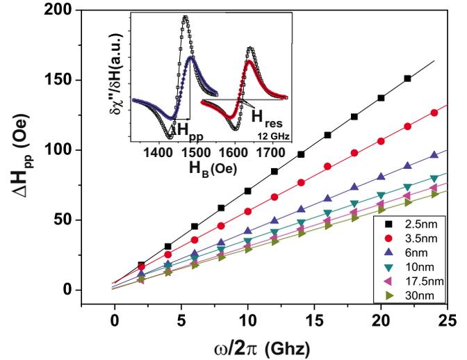
FIG. 2. (Color online) Frequency-dependent peak-to-peak FMR linewidth  $\Delta H_{pp}(\omega)$  for FM =  $\text{Ni}_{81}\text{Fe}_{19}$ ,  $t_{FM}$  as noted, films with Pt overlayers. *Inset*: Lineshapes and fits for films with (filled circles) and without (open squares) Pt overlayers, FM =  $\text{Ni}_{81}\text{Fe}_{19}$  (right), CoFeB (left).
