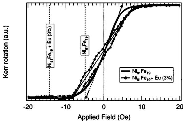
FIG. 5. MOKE hard-axis hysteresis loops for undoped and Eu-doped  $\text{Ni}_{81}\text{Fe}_{19}$ ; dynamic  $H_k$  values are shown for comparison.
