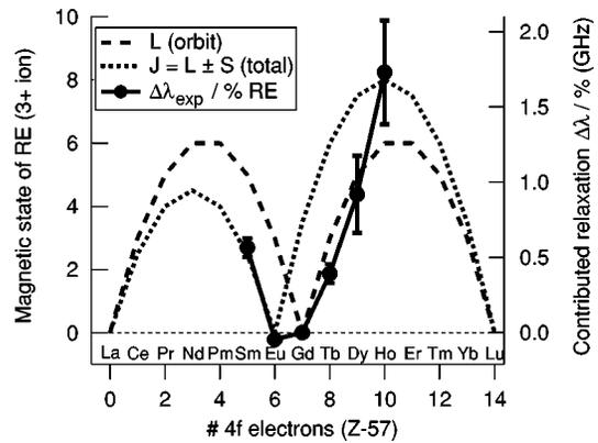
FIG. 3. Contributed damping to  $Ni_{81}Fe_{19}$  as a function of lanthanide dopant atomic number  $Z-57$  ( $La=57$ ). The angular momentum states of the isolated dopants are shown for comparison.
