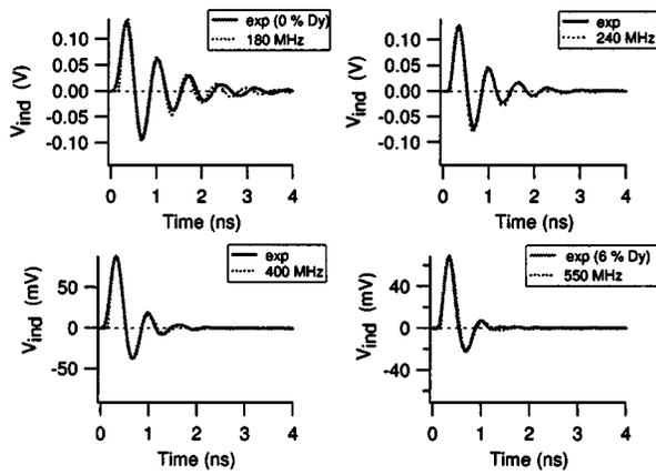
FIG. 1. Inductive response [voltage  $V_{ind}(t)$ ] for a series of Dy-doped  $Ni_{81}Fe_{19}$  films, increasing doping  $0\% < x_{Dy} < 6\%$ . LL/LLG fits and estimated values of  $\lambda/4\pi$  are shown. There is an evident increase in relaxation rate  $\lambda$  with composition, spanning  $180 < \lambda/4\pi < 550$  MHz ( $0.014 < \alpha < 0.043$ ).
