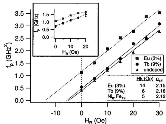
FIG. 4. Kittel plot for undoped, Tb-doped, and Eu-doped  $Ni_{81}Fe_{19}$ , longitudinal bias. Inset, left:  $\omega_p$  vs bias field  $H_B$ . Table, right: extracted values of dynamic  $H_K$  and  $g$ -factor. Note the 9 Oe enhancement of dynamic  $H_K$  provided by Eu.
