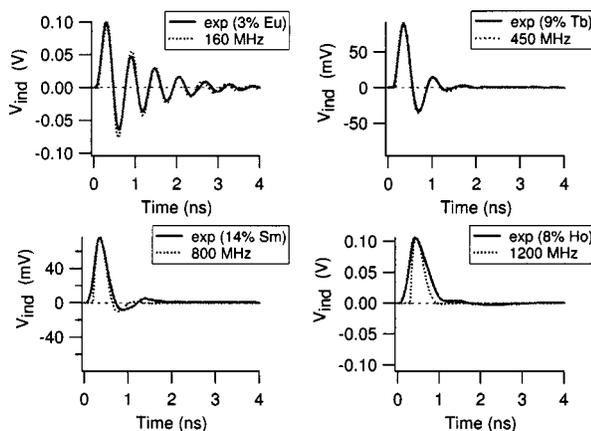
FIG. 2. Comparable fits for representative members of the Eu, Sm, Tb, and Ho series, with composition characterized by XPS. Strong effects on damping are observed for all dopants except Eu.
