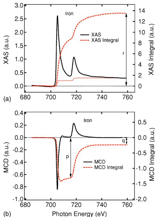
FIG. 1. (Color online)  $L_{2,3}$ -edge XAS and MCD spectra of iron at undoped  $\text{Ni}_{81}\text{Fe}_{19}$  thin film: (a) summed XAS spectra and its integral; (b) MCD spectra and its integral.
