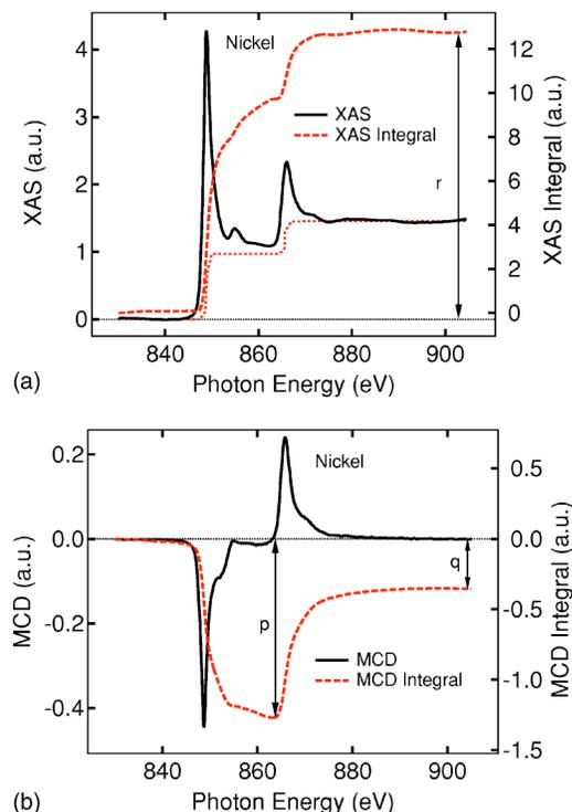
FIG. 2. (Color online)  $L_{2,3}$ -edge XAS and MCD spectra of nickel at undoped  $\text{Ni}_{81}\text{Fe}_{19}$  thin film: (a) summed XAS spectra and its integral; (b) MCD spectra and its integral.
