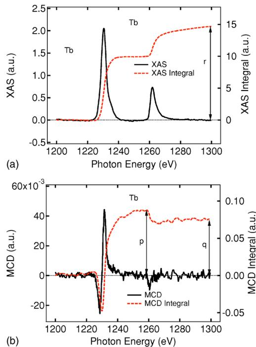
FIG. 3. (Color online)  $M_{4,5}$ -edge XAS and MCD spectra of Tb at 6% Tb-doped  $\text{Ni}_{81}\text{Fe}_{19}$  thin film: (a) summed XAS spectra and its integral; (b) MCD spectra and its integral.
