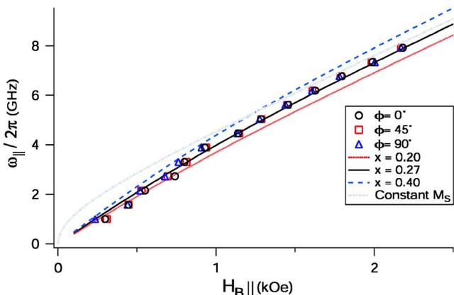
FIG. 3. (Color online) Resonance frequencies  $\omega_{\parallel}(H_B)$ , for different field orientations  $\phi$ , in-plane (pc) configuration, from Fig. 2, left. Model calculations for thin-film superparamagnetic resonance [Eq. (1)], varying volume fraction  $x$  from TEM-measured  $x=0.27$ . See text for details.
