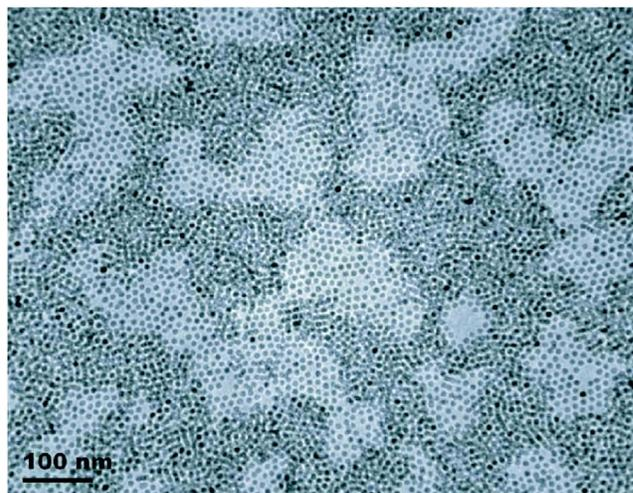
FIG. 1. (Color online) TEM image of 1–2 monolayers of  $7.5 \pm 0.8$  nm  $\gamma\text{-Fe}_2\text{O}_3$  nanoparticles. Light and dark regions correspond to single- and double-monolayer regions, respectively. Local hexagonal ordering is clearly seen; an average center-to-center spacing of 10.5 nm is identified in one-monolayer regions.
