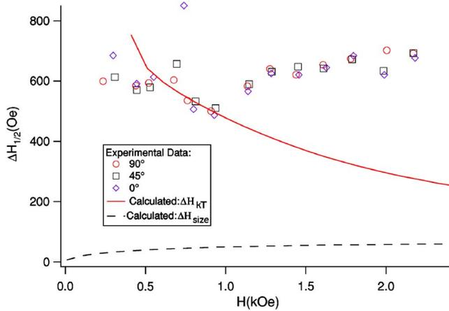
FIG. 5. (Color online) Swept-field peak-to-peak linewidths  $\Delta H_{pp}(\omega)$  for the pc resonance data in Fig. 2, left. The calculated effects of 10% dispersions in SP NC size  $\Delta H_{size}(\omega)$  and coverage  $\Delta H_K(\omega)$  are indicated with anisotropy field dispersion  $\Delta H_K$ . See text for details.
