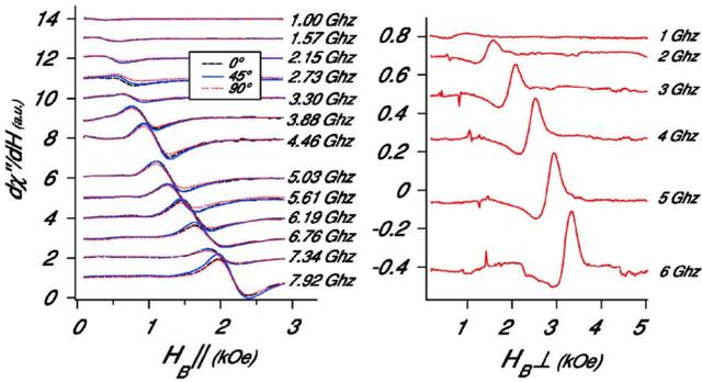
FIG. 2. (Color online) Broadband FMR measurements of 7.5 nm SP  $\gamma$ -Fe<sub>2</sub>O<sub>3</sub> thin film. Left: pc measurements of  $\omega_{\parallel}$ , for field  $H_B$  orientations of 0, 45, and 90° to sample flat. Right: nc measurements of  $\omega_{\perp}$ . See text for details.
