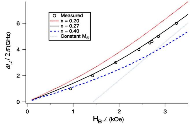
FIG. 4. (Color online) Resonance frequencies  $\omega_{\perp}(H_B)$  for normal configuration (nc), calculated according to Eq. (1), as in Fig. 2.
